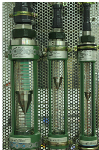
Figure 3.3: Rotameters to control the flow rate.
