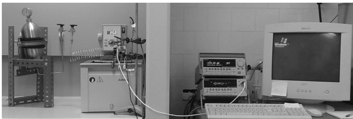
Figure 3.2: Schematic of the experimental setup. (A) 1 liter expansion vessel, (B) coiled tubing, (C) thermostatic bath, (D) data acquisition system, (E) computer
