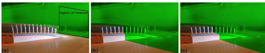
Figure 5.12. The laser sheet arrangements for the vertical plane analysis: (a) behind the heat exchanger; (b) on the 6 th fin; (c) between the 6 th and 7 th fins, in the middle of the heat exchanger.
