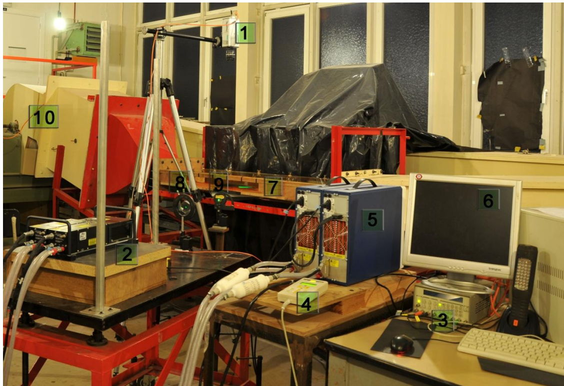
Figure 5.4. The second PIV experimental set-up: 1.Camera, 2.Nd-YAG green laser, 3.Synchroniser, 4.Wired remote control for laser, 5.Laser twins' box, 6.Computer, 7.Test section, 8.Focal lens, 9.Cylinder lens, 10.Particle introduction.
